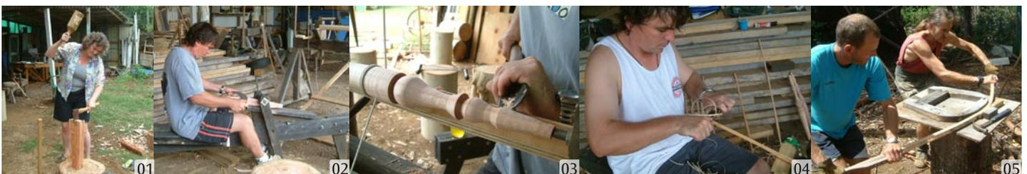
shaping the seat by hand using an adze, in-shaves and scrapers.
